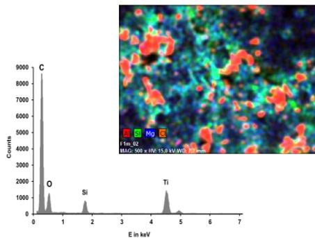
X-ray spectra give quantitative information about the elemental composition of the sample surface. 1D scans and 2D maps can be generated.
